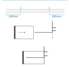
For cavity barriers 91mm-215mm wide (across cavity) use 2 MP brackets and the 160mm long spike. The 160mm spike will require cutting to size, if used in barriers less than 185mm wide, to ensure that the spike does not pierce through the face of the intumescing material, the bracket should be cut to provide a minimum projection through the barrier to 3/4 of the cavity barrier width and to a maximum of 25mm behind the face of the intumescing strip.
