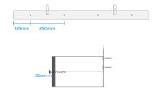
Screw the pigtail screws through the face of the intumescing material on the face of the cavity barrier (the face with the labels).
