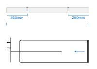
Fix 2 number HP brackets, per linear meter, to the substrate at maximum 250mm from the end of the cavity barrier, with a maximum spacing between brackets of 500mm.
