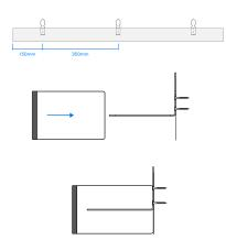
Fix 3 number MP brackets, per linear meter, to the substrate at maximum 150mm from the end of the cavity barrier, with a maximum spacing between brackets of 350mm.
